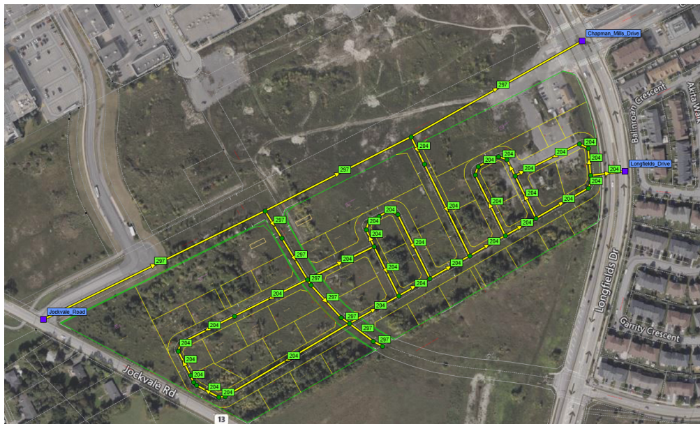
Figure 3.1 Proposed Watermain Layout and Pipe Diameters (mm)
