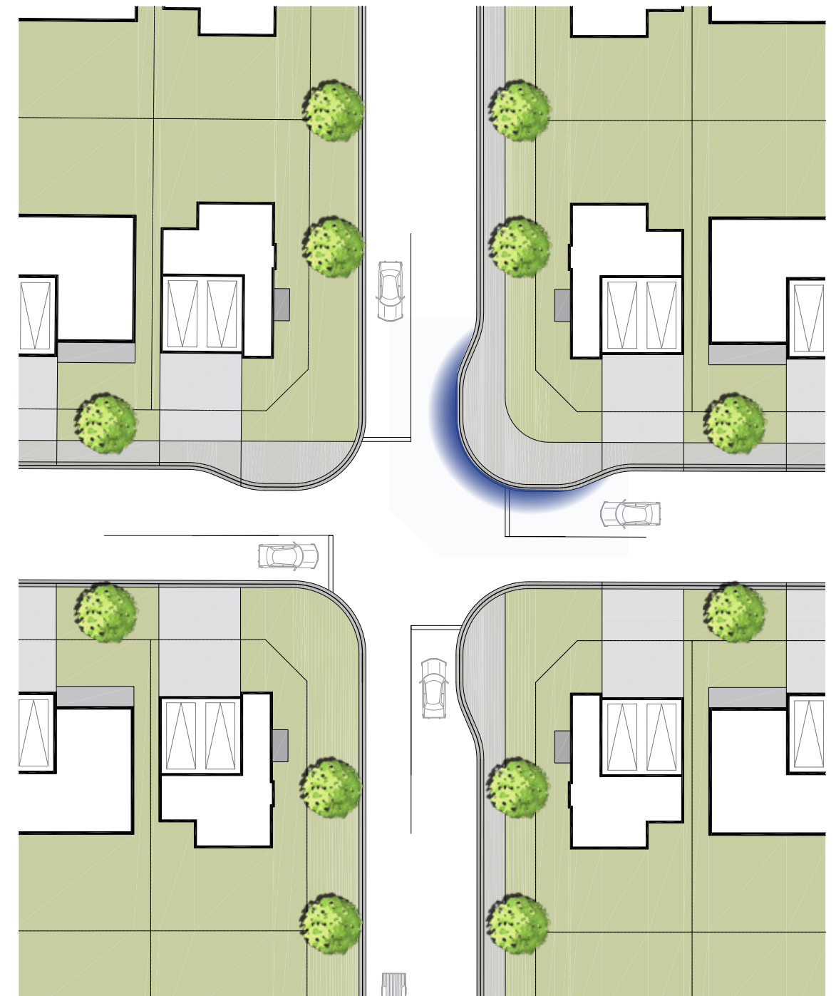
Figure 40 Double Bulb-Out at Intersection
