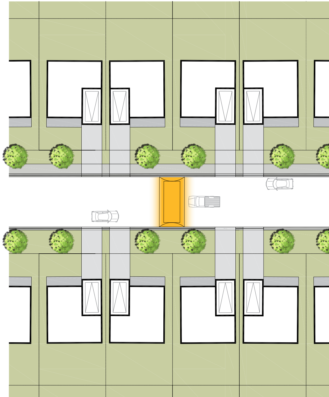
Figure 41 Speed Hump on Local Road
