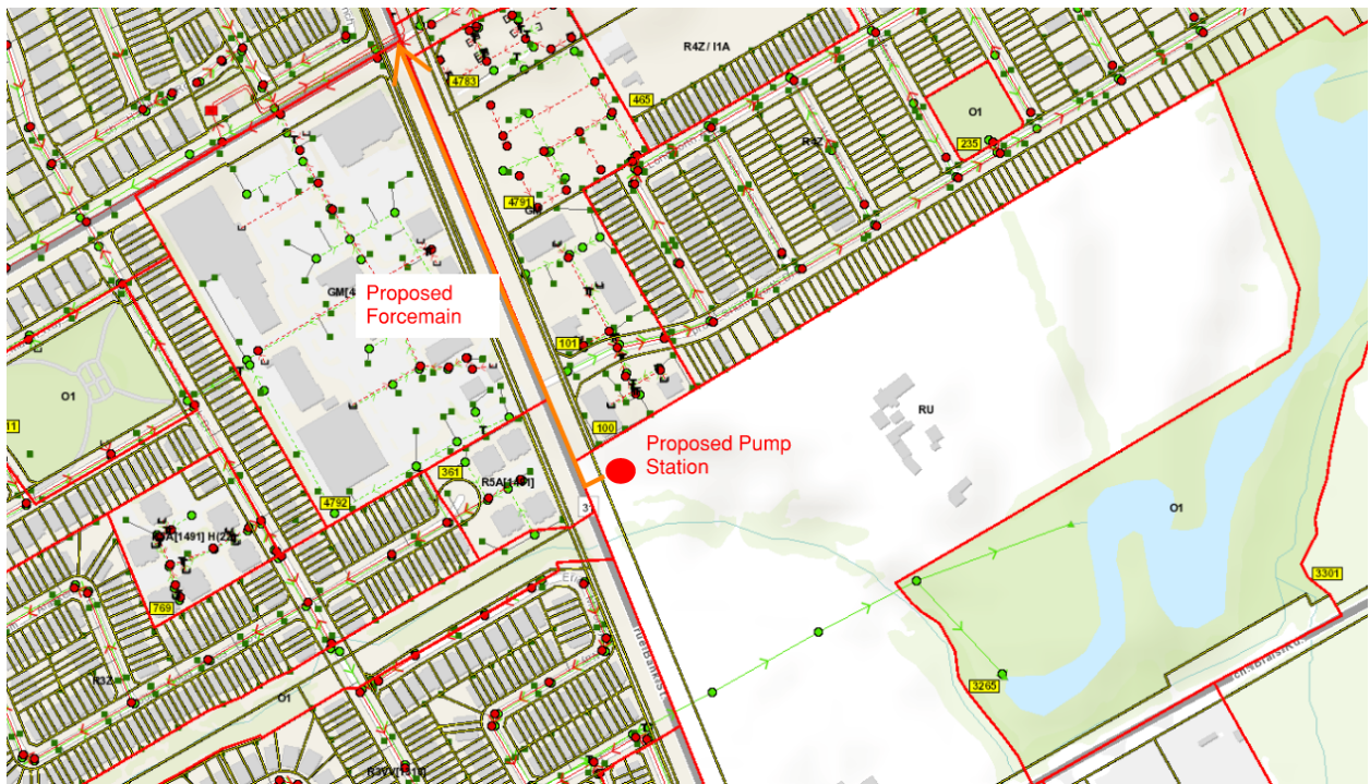
Figure 1 – Proposed Pump Station
