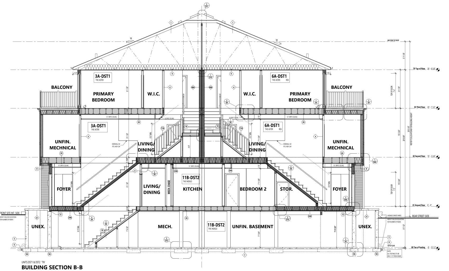
**ROOF FRAMING:** ALL LAMINATED VENEER LUMBER (LVL) BEAMS, BUILT-UP BEAMS, GIRDER TRUSSES AND METAL HANGER CONNECTIONS SUPPORTING ROOF FRAMING TO BE DESIGNED AND CERTIFIED BY ROOF TRUSS MANUFACTURER. REFER TO ROOF TRUSS SHOP DRAWINGS FOR ALL ROOF FRAMING INFORMATION UNLESS OTHERWISE NOTED ON
