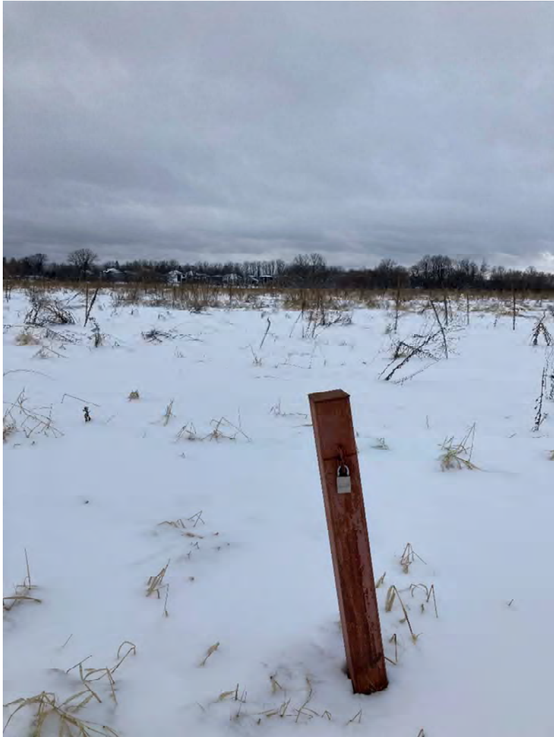
Photograph 3 – One of several monitoring wells identified across the Site.
