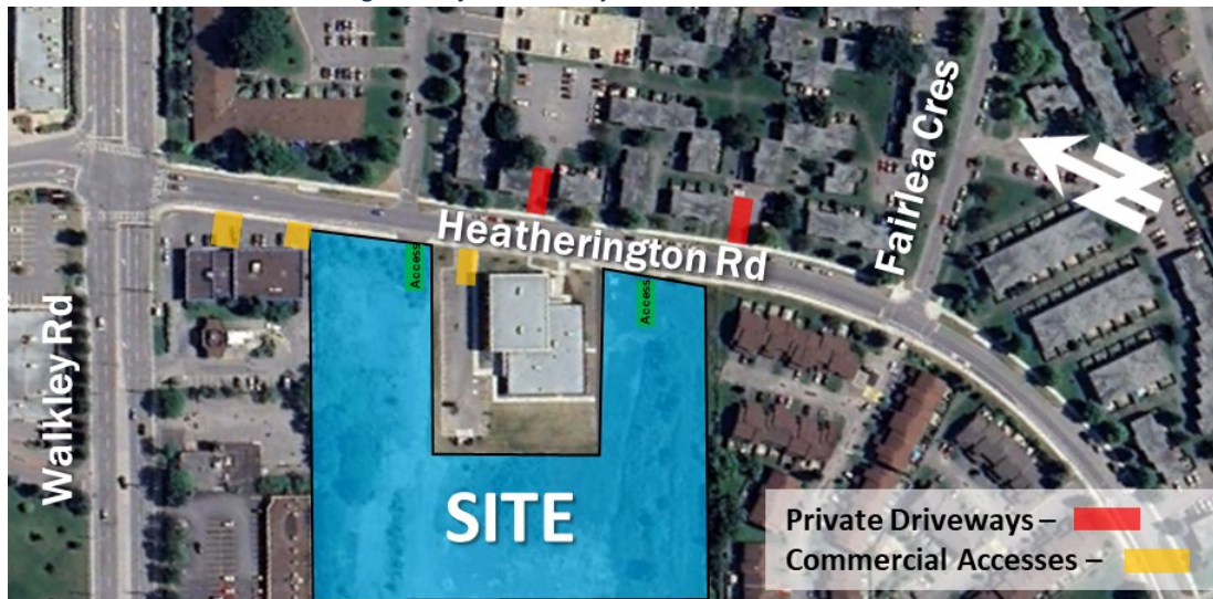
Figure 3: Adjacent Driveways within 200m of Site Access
