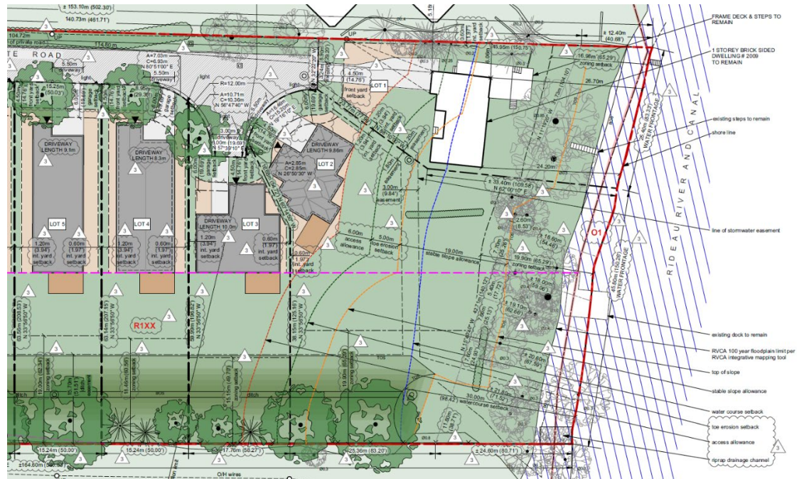
Figure 27: Subject site stable slope allowance and watercourse setback.
