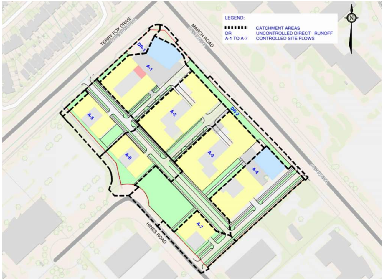
Figure 6: Conceptual Stormwater Management Plan
