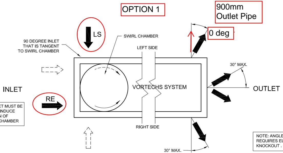
NOTE: DUAL INLET MUST BE POSITIONED TO INDUCE SAME DIRECTION OF FLOW IN SWIRL CHAMBER
