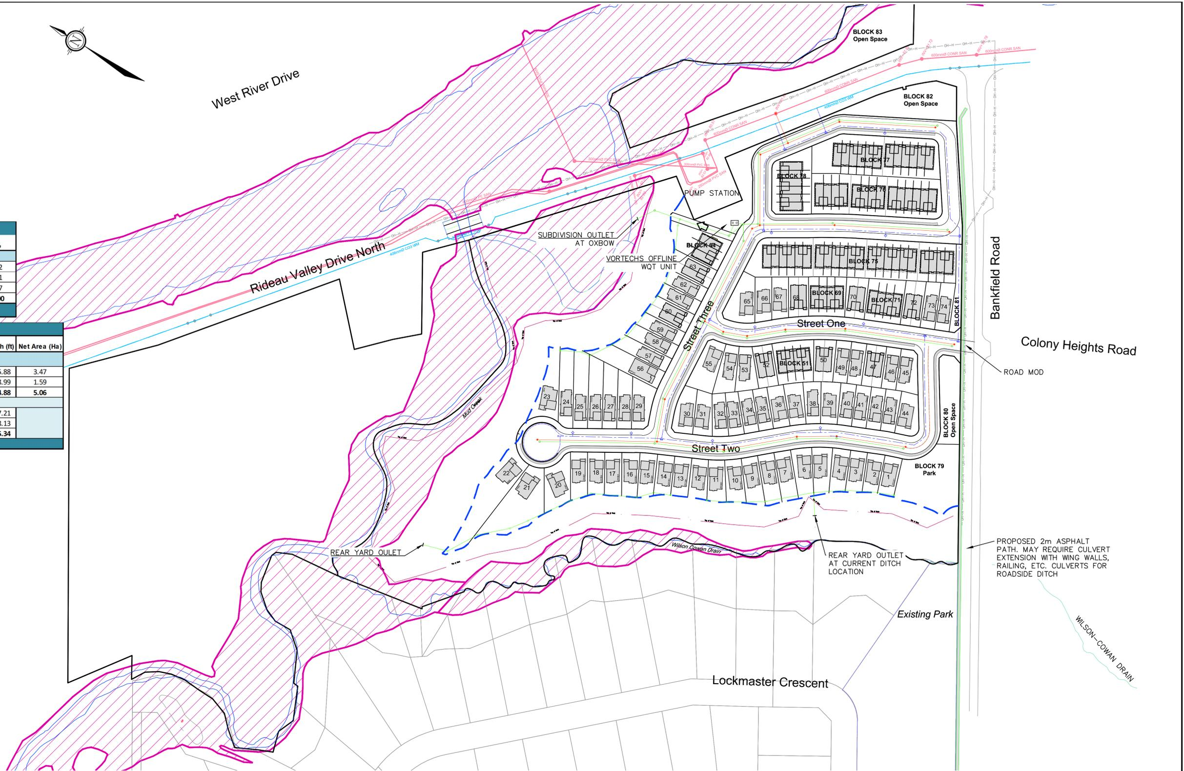
PROPOSED 2m ASPHALT PATH. MAY REQUIRE CULVERT EXTENSION WITH WING WALLS, RAILING, ETC. CULVERTS FOR ROADSIDE DITCH
