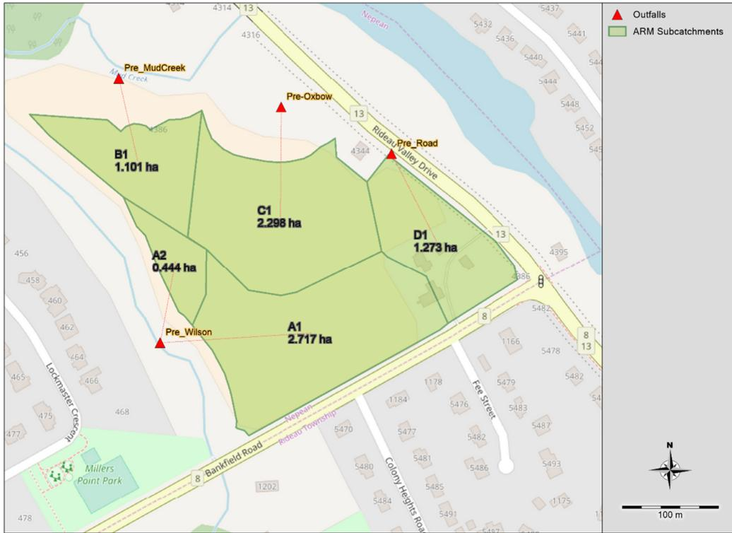
**Figure 1: PCSWMM Model Schematic – Existing conditions**
