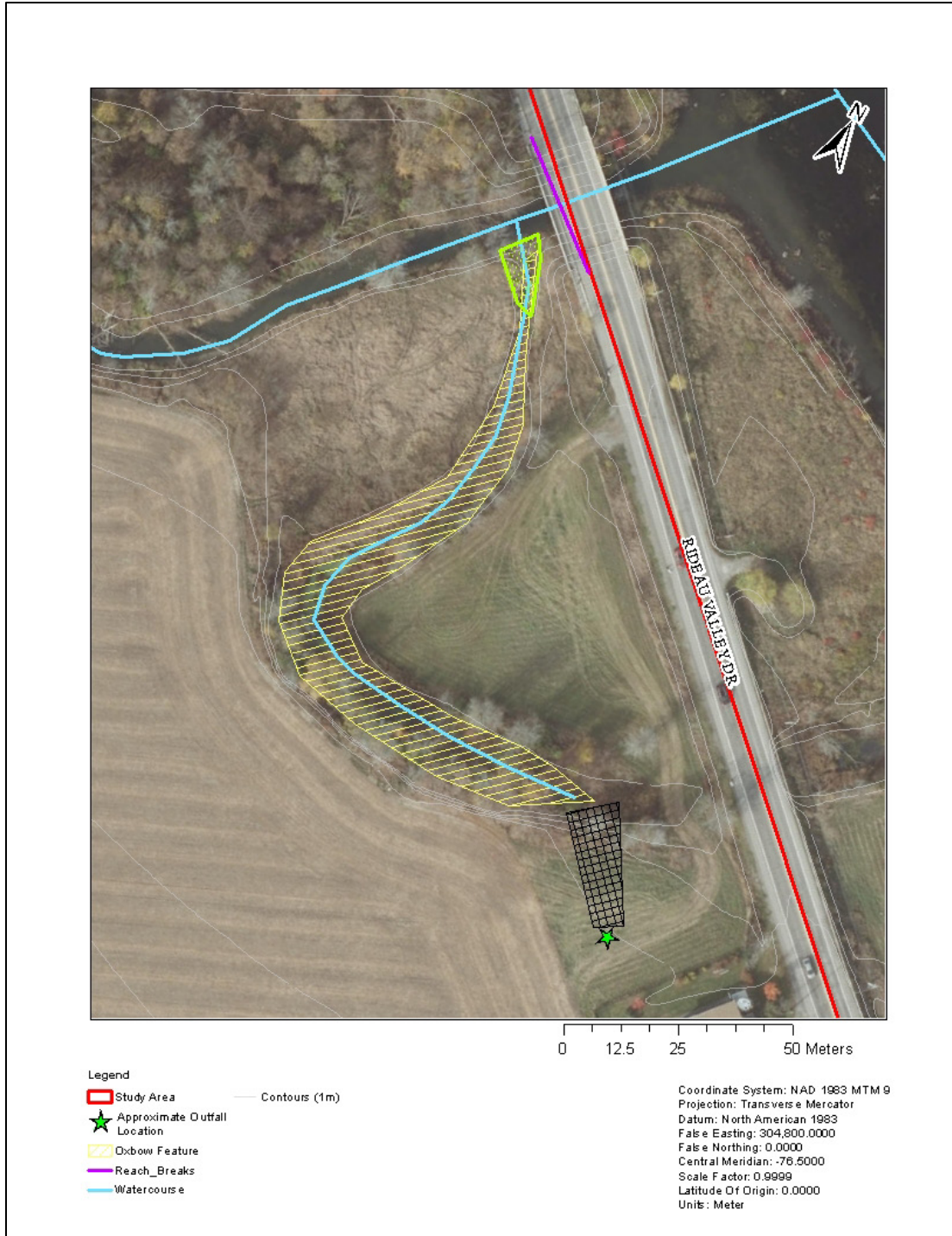
FIGURE 8 Recommended Design Opportunities for Stormwater Management Outflows
