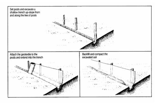
Figure 5: Typical installation of silt fences
