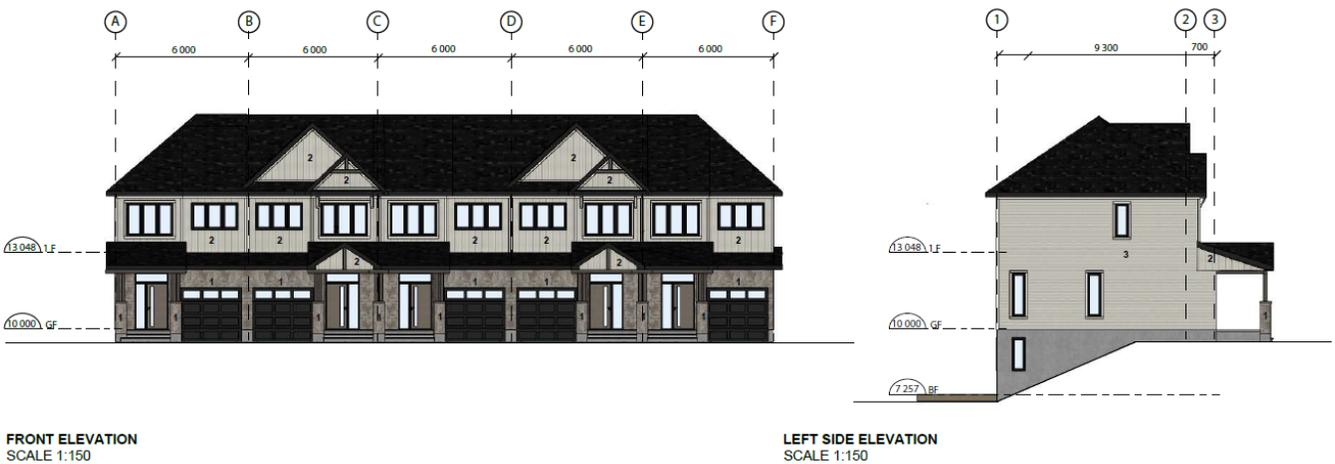
Figure 13. Front and left side elevation of Townhouse Model 4 - "E" (private lane).
