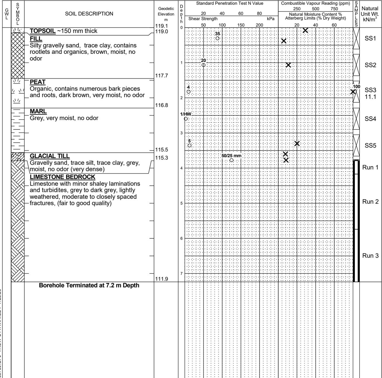
LOG OF BOREHOLE BH LOGS - 258780.GPJ TROW OTTAWA.GDT 7/23/20
