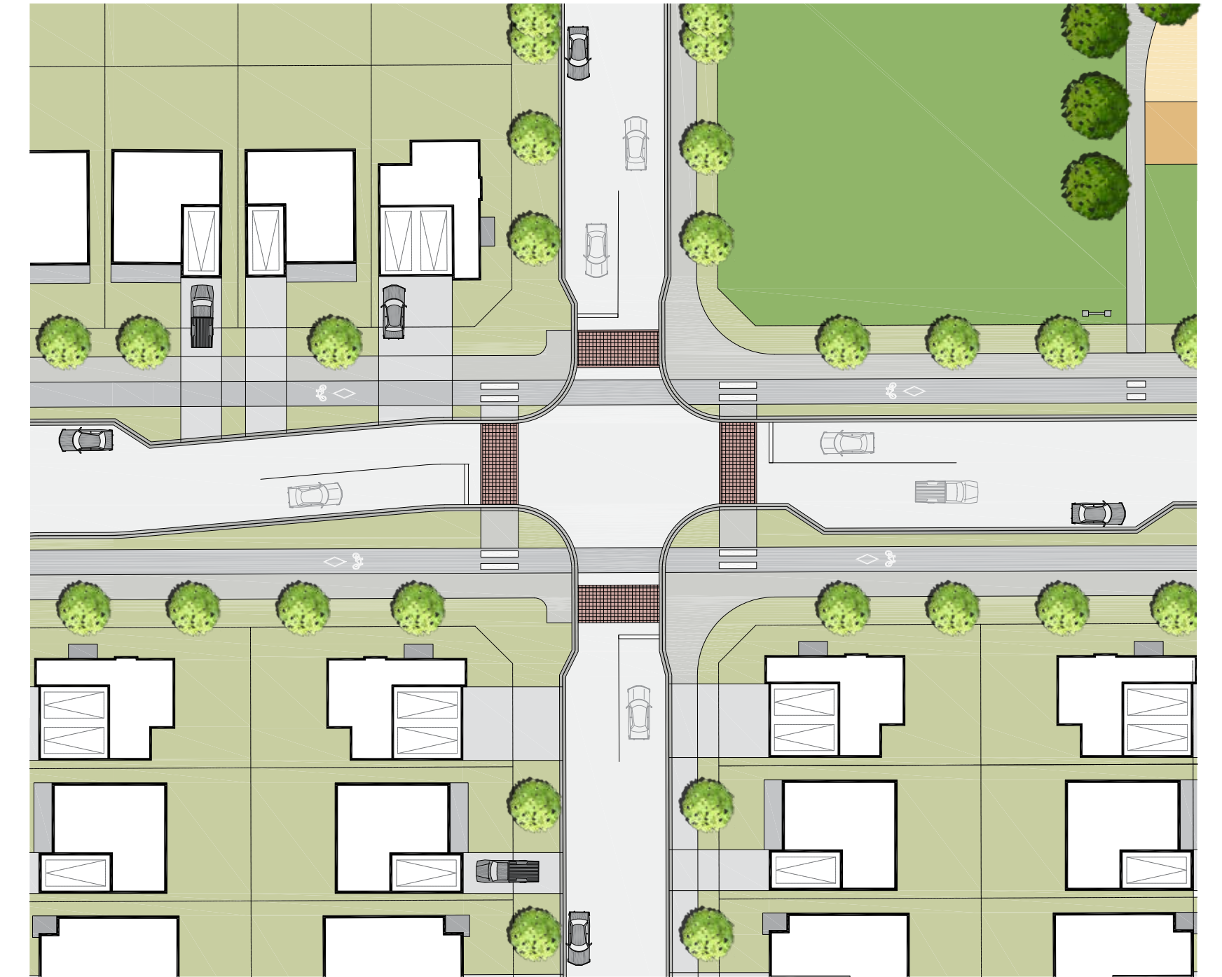
Figure 52 Double Bulb-Out at Collector Road and Local Road Intersection
