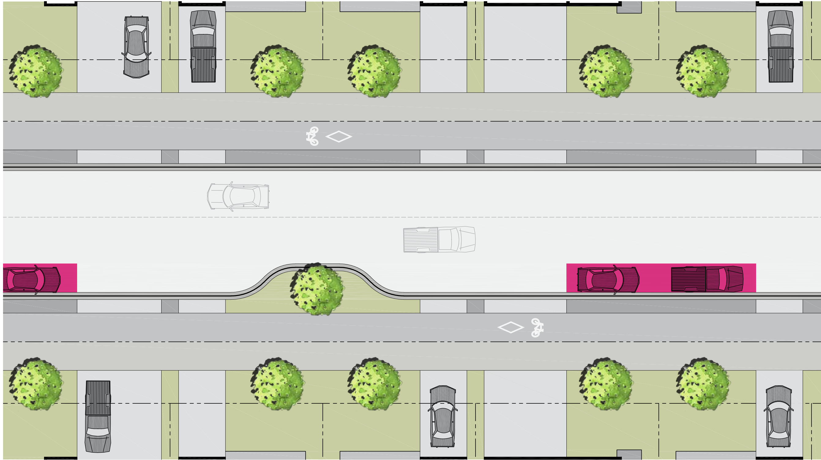
Figure 45 On-Street Parking Demonstration on Collector Road
