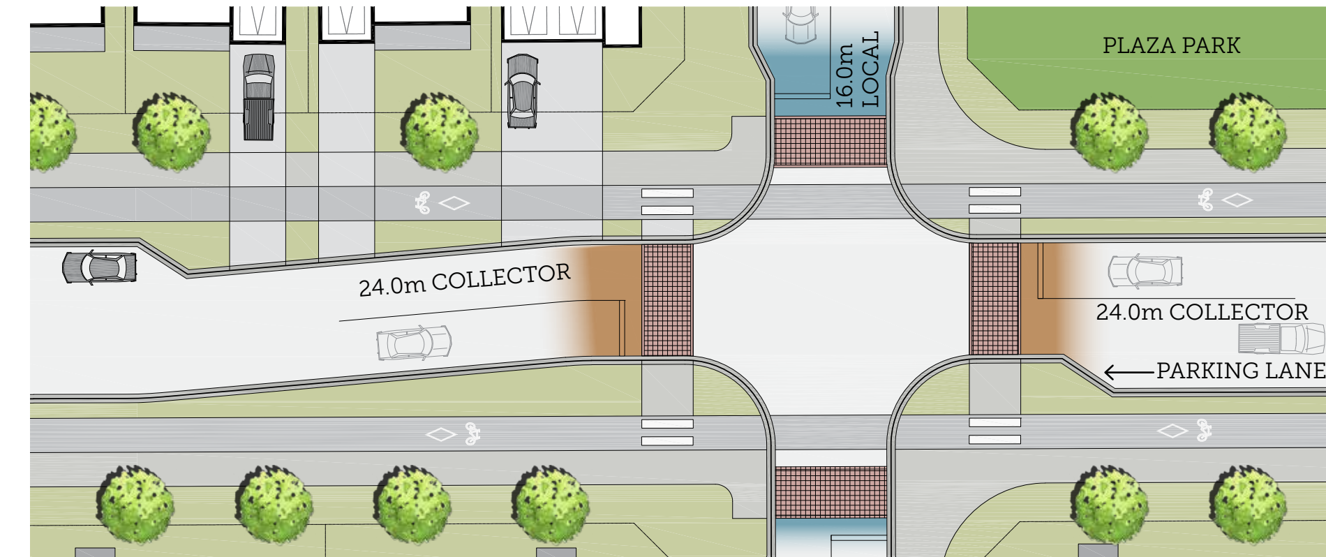
Figure 35 Intersection of 24.0m Collector Road with 16.0m Local Road
