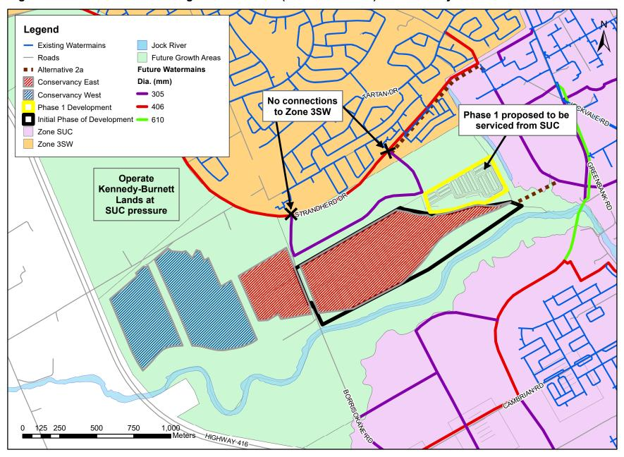
Figure 2: Alternative 2a - Servicing from Zone SUC (from Strandherd) w/ Secondary Feed from NTC
