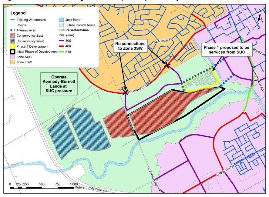
Figure 4: Alternative 2c - Servicing from Zone SUC (from NTC) w/ Secondary Feed from NTC
