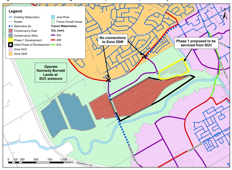
Figure 3: Alternative 2b - Servicing from Zone SUC (from Strandherd) w/ Secondary Feed from Barrhaven South
