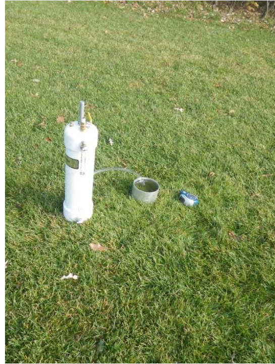
Figure 3: Single Ring Infiltrrometer Setup (12.7 cm diameter steel ring, single Marriotte bottle)
