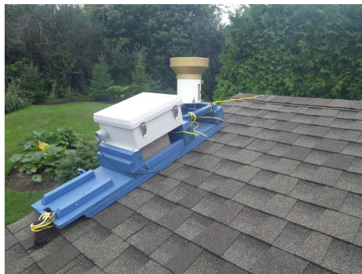
Figure 2e: Rain gauge installation
