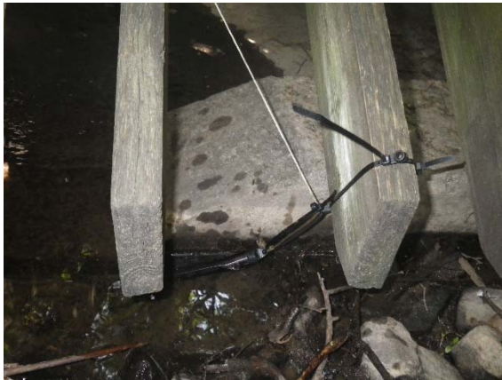
Figure 2c: Water level logger installation at Q3
