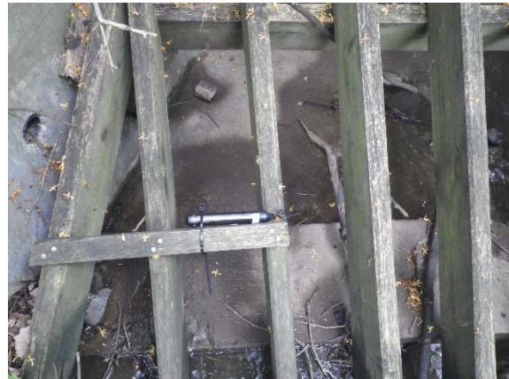
Figure 2d: Barometric Logger Installation at Q3
