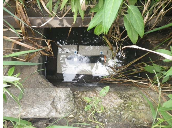
Figure 2b: Water level logger installation at Q2
