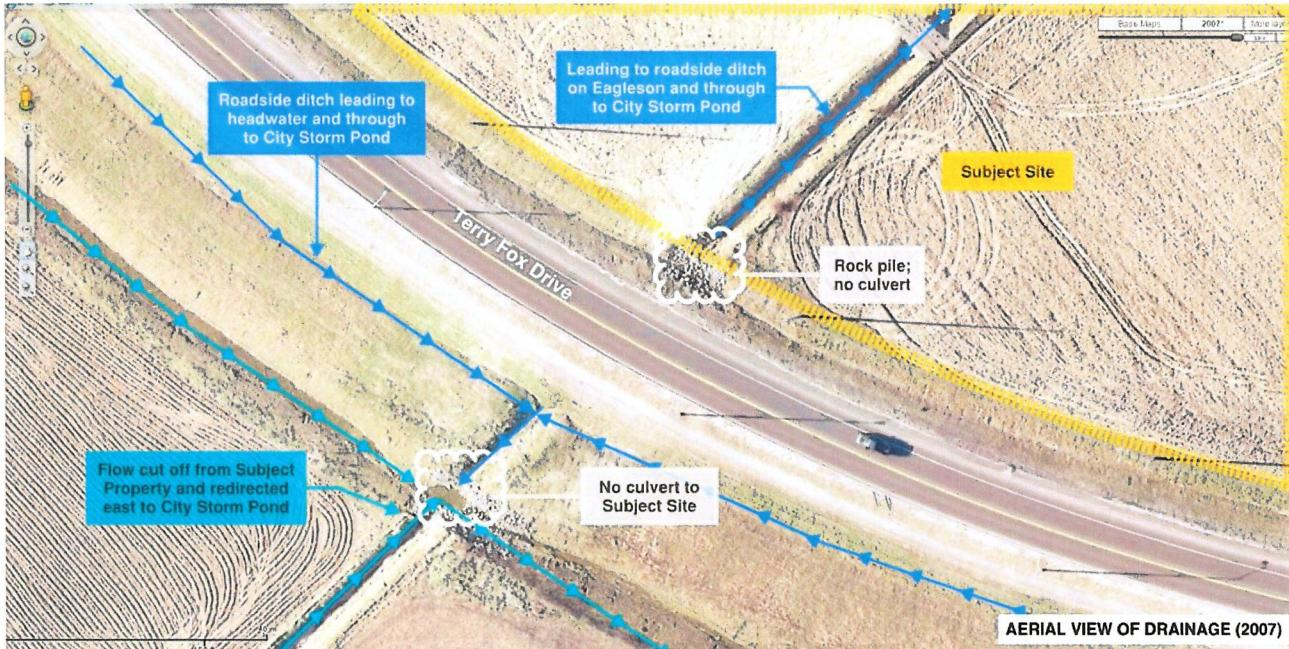
Figure 1: Drainage Patterns on and Around Subject Site
