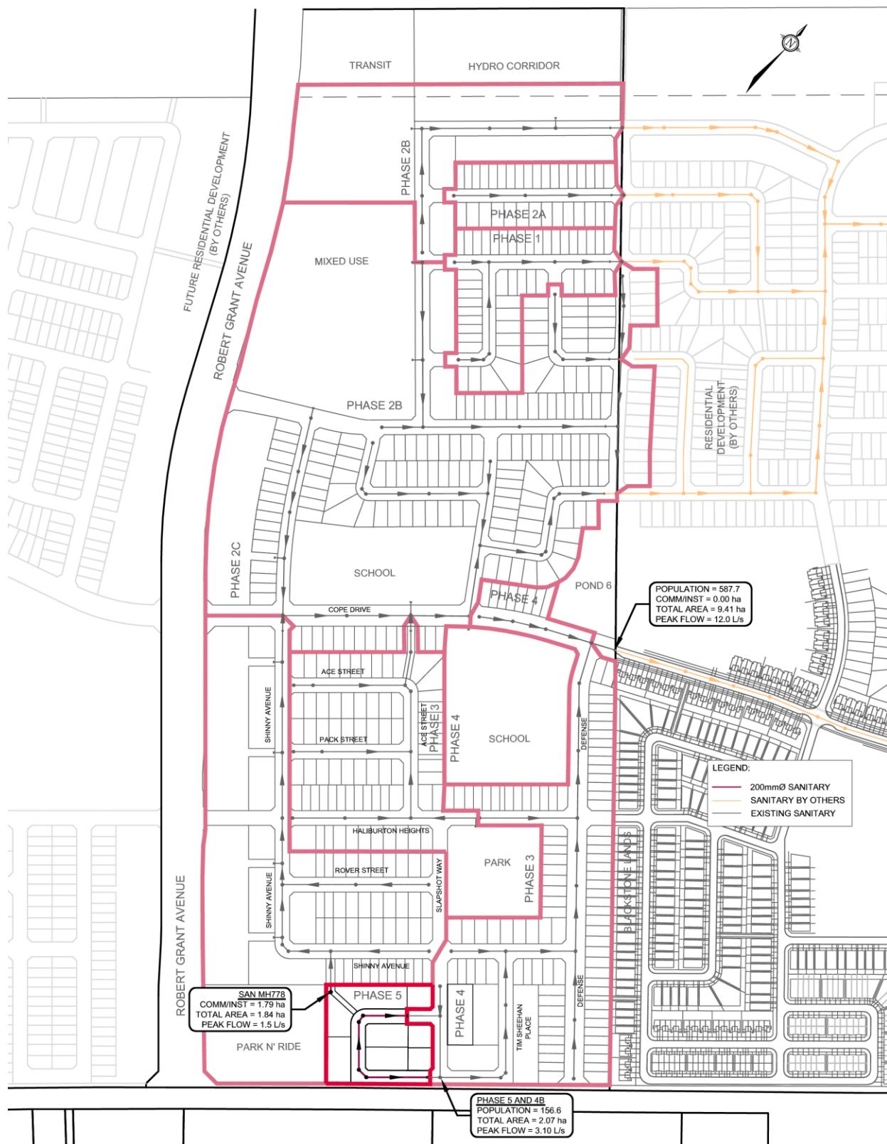
**Figure 4: Sanitary Sewer Network**
