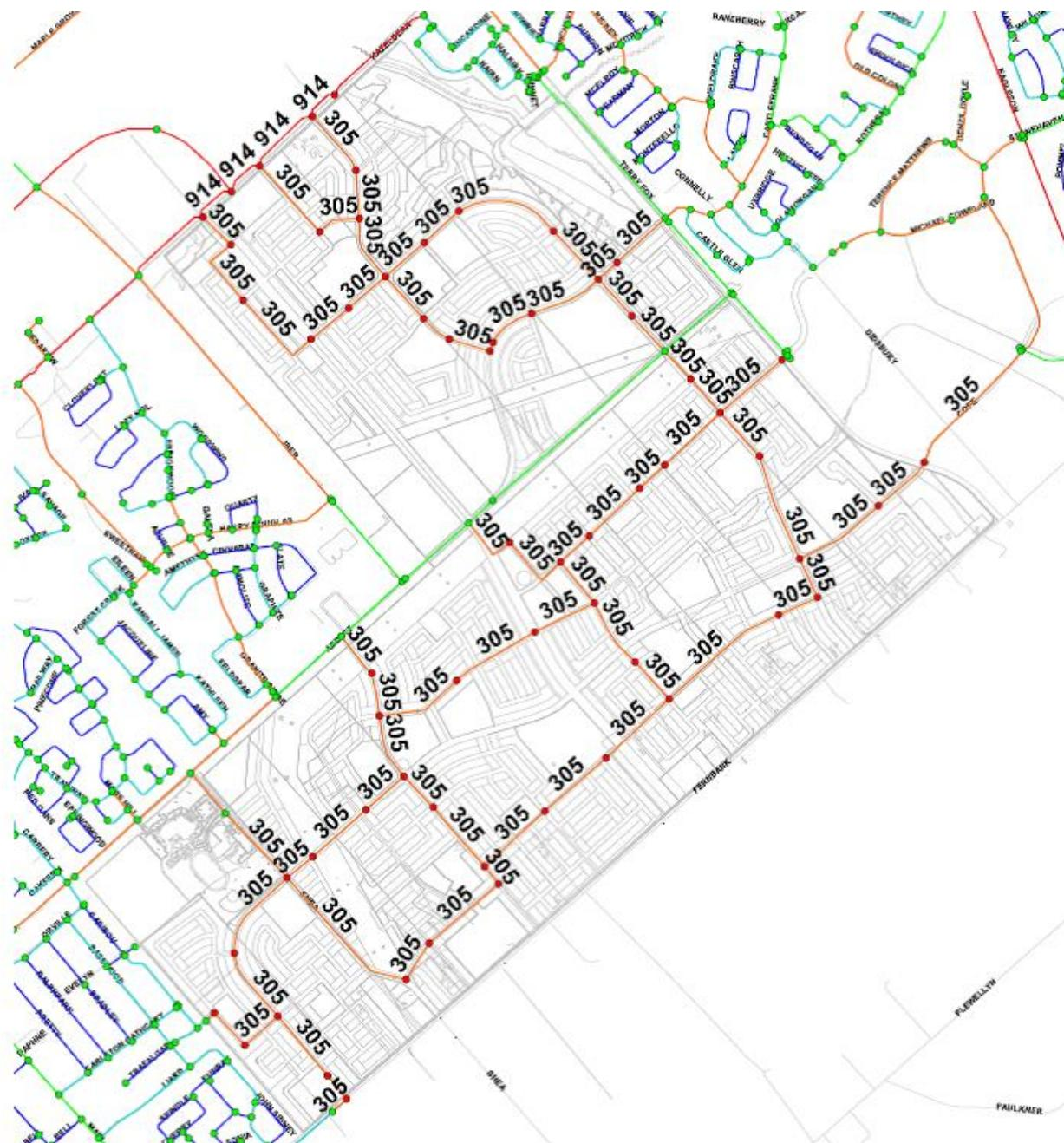
Figure 7: Build-out watermain alignment and sizing (Figure A-5 from MSS [2])
