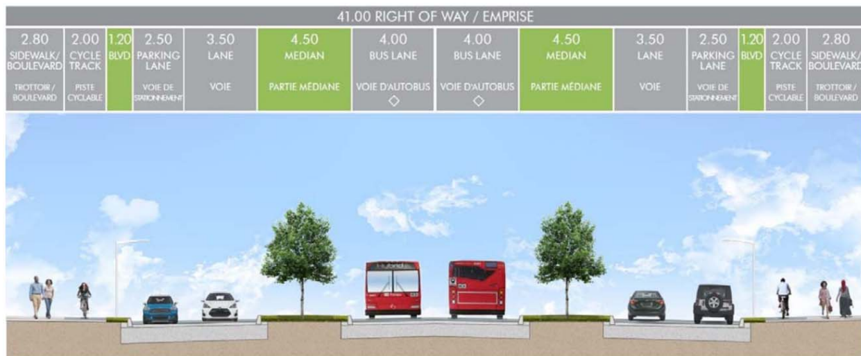
Figure 6: Chapman Mills Drive Future Cross Section
