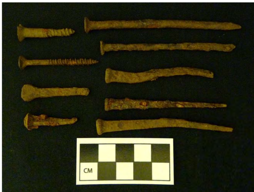
Image 64: Example of metal hardware (clockwise from bottom left): wrought nail, horseshoe nail, Robertson screw, slot screw, wire nails (2), machine cut nails (3).
