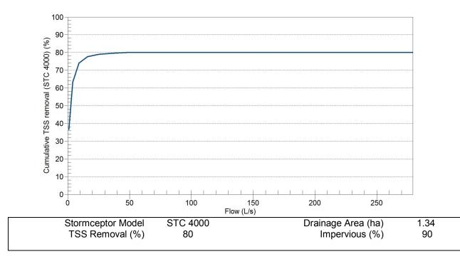
**Figure 3.** Cumulative TSS Removal by Flow Rate for OTTAWA MACDONALD-CARTIER INT'L A – 6000, 1967 to 2003. Stormceptor continuously removes TSS throughout the full range of storm events analyzed. Note that large events do not significantly impact the average annual TSS removal. Therefore no decline in cumulative TSS removal indicates scour does not occur as the flow rate increases.
