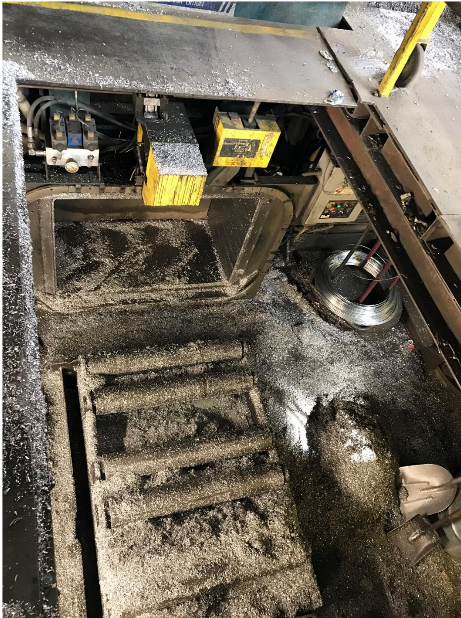
Photograph 5: View of the open hydraulic bailer chamber on the top of the photo, the rollers located on the bottom of the photograph raise up to the warehouse floor for removal of the bailed metal (August 2019)
