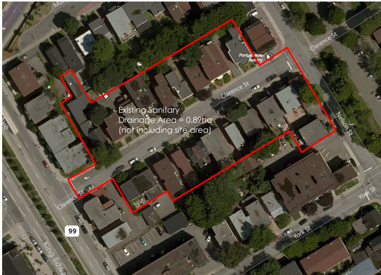
Figure 2: Existing Sanitary Drainage Area
