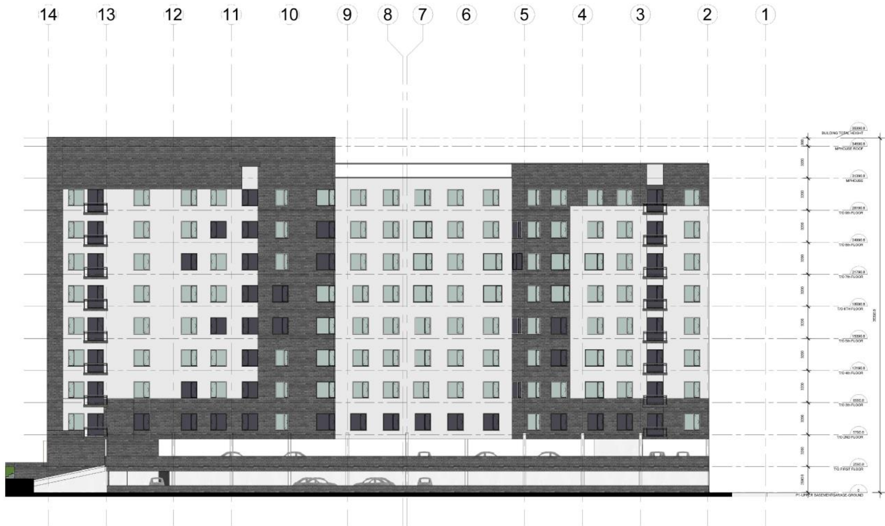
Figure 12. Proposed east elevation prepared by Roderick Lahey Architect Inc.
