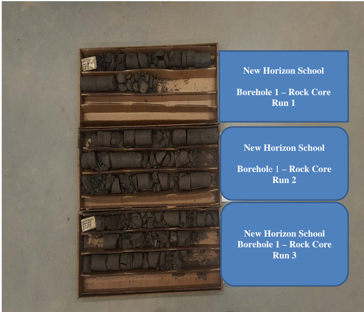
Photo No. B5: Bedrock Cores from Borehole No. 1 –Run 1, Run 2 and Run 3
