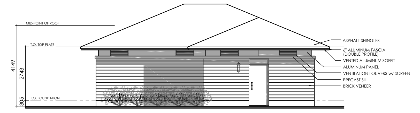
8 ACCESSORY BUILDING - SIDE ELEVATION A1 SCALE: 1:100
