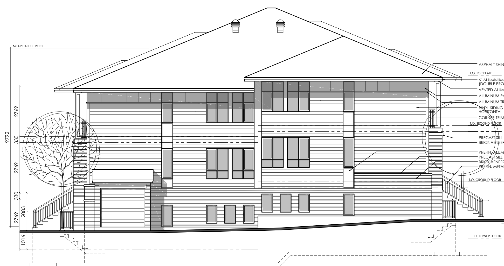
6 STEPPED BUILDING - SIDE ELEVATION A1 BLOCKS 3,4,5,6 SCALE: 1:100
