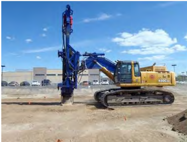
Photo 1: Rapid Impact Compaction Equipment (Source: Menard Canada)
