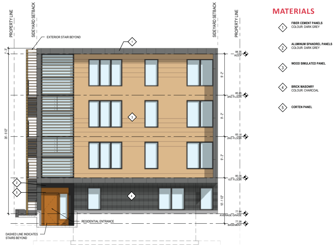
FIG.16 PROPOSED SOUTH-WEST ELEVATION
