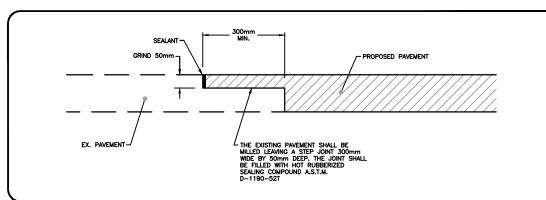
MEDIAN/STEP JOINT DETAIL SCALE: N.T.S.
