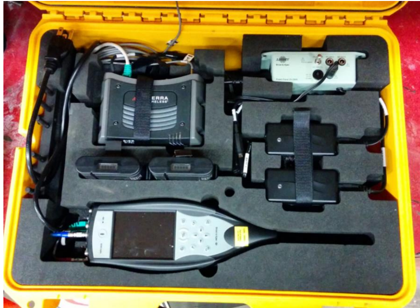
PHOTOGRAPH 2: INTERNAL COMPONENTS OF NOISE MONITORING STATION
