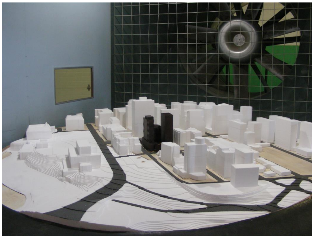
PHOTOGRAPH 1: STUDY MODEL INSIDE THE GWE WIND TUNNEL LOOKING DOWNWIND
