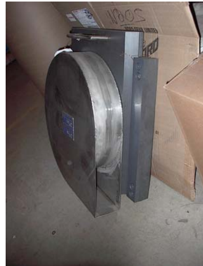
FV-VHV (mounted on sliding plate for emergency bypass)
