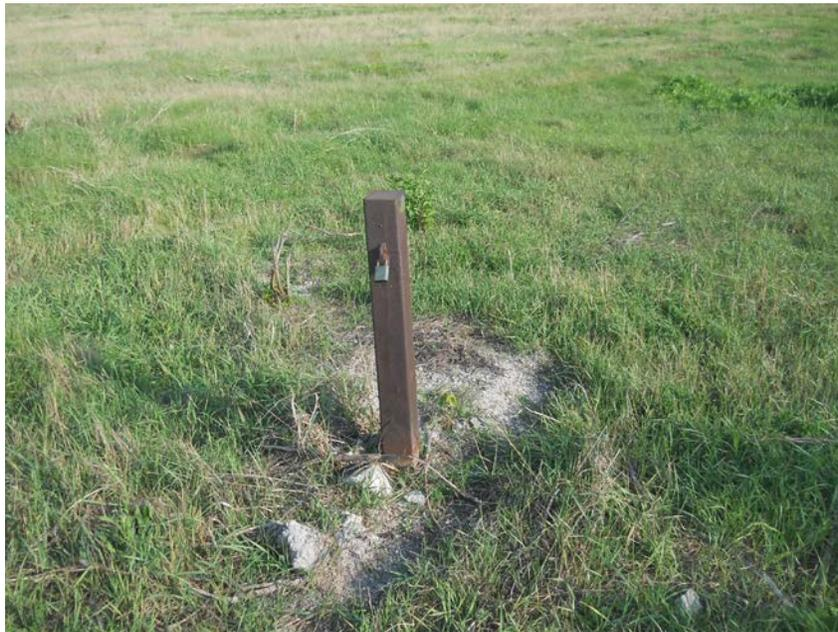
Photo 7: View of a typical monitoring well on the Site.
