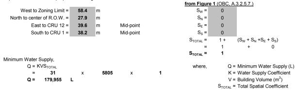
The governing water supply for fire protection considering all non-sprinklered buildings on-site is,
