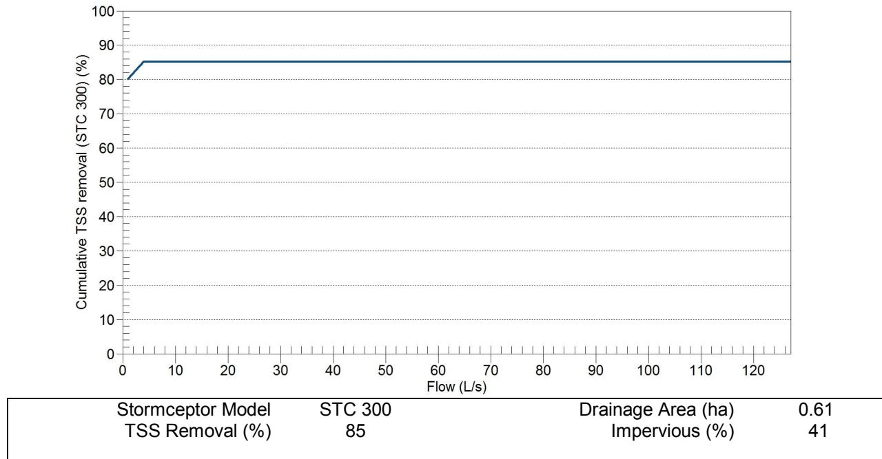
**Figure 3. Cumulative TSS Removal by Flow Rate for OTTAWA MACDONALD-CARTIER INT'L A – 6000, 1967 to 2003.** Stormceptor continuously removes TSS throughout the full range of storm events analyzed. Note that large events do not significantly impact the average annual TSS removal. Therefore no decline in cumulative TSS removal indicates scour does not occur as the flow rate increases.
