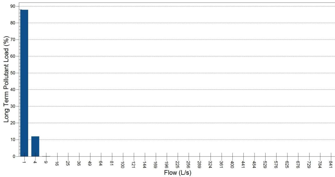
**Figure 2. Long Term Pollutant Load by Flow Rate for OTTAWA MACDONALD-CARTIER INT'L A – 6000, 1967 to 2003 for 0.61 ha, 41% impervious.** The majority of the annual pollutant load is transported by small frequent storm events. Conversely, large infrequent events carry an insignificant percentage of the total annual pollutant load.
