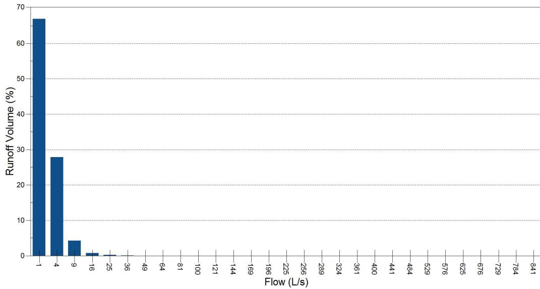
**Figure 1. Runoff Volume by Flow Rate for OTTAWA MACDONALD-CARTIER INT'L A – ON 6000, 1967 to 2003 for 0.61 ha, 41% impervious.** Small frequent storm events represent the majority of annual rainfall volume. Large infrequent events have little impact on the average annual TSS removal, as they represent a small percentage of the total annual volume of runoff.
