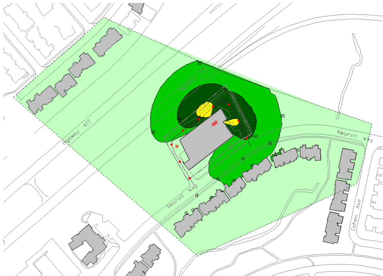
FIGURE 4: PREDICTED NIGHTTIME OUTDOOR NOISE LEVELS (AHU UNITS ONLY)
