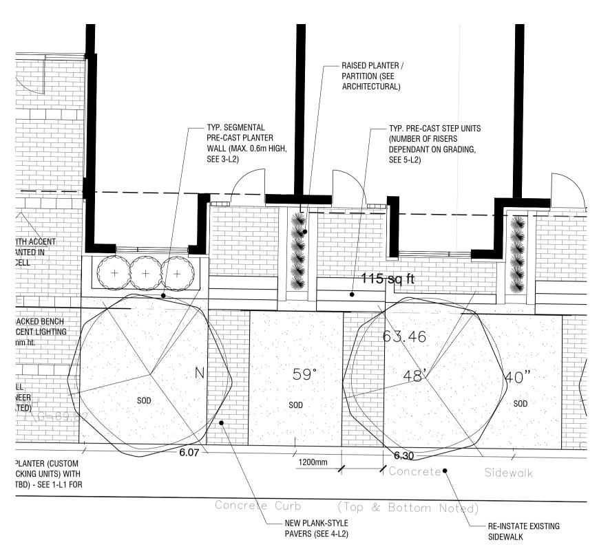
GATE – 2.13m High wood Privacy fe∰e (SEE 6-L2) 100 sq ft TYP. PRE-CAST CONCRETE STEP RISERS (SEE 5-L2) EXISTING TREE TO BE RETAINED (CRZ INDICATED) - SEE TCR FOR PROTECTION 1.50 -**DETAILS** CAREFULLY REMOVE EXISTING TOPSOIL WITHOUT DISTURBING TREE ROOTS AND **INSTALL Stabilized Decomposed Granite** PATHWAY DIRECTLY ON SUB-GRADE. - NEW PLANK-STYLE - EXISTING CONCRETE CURB TO BE REMOVED
