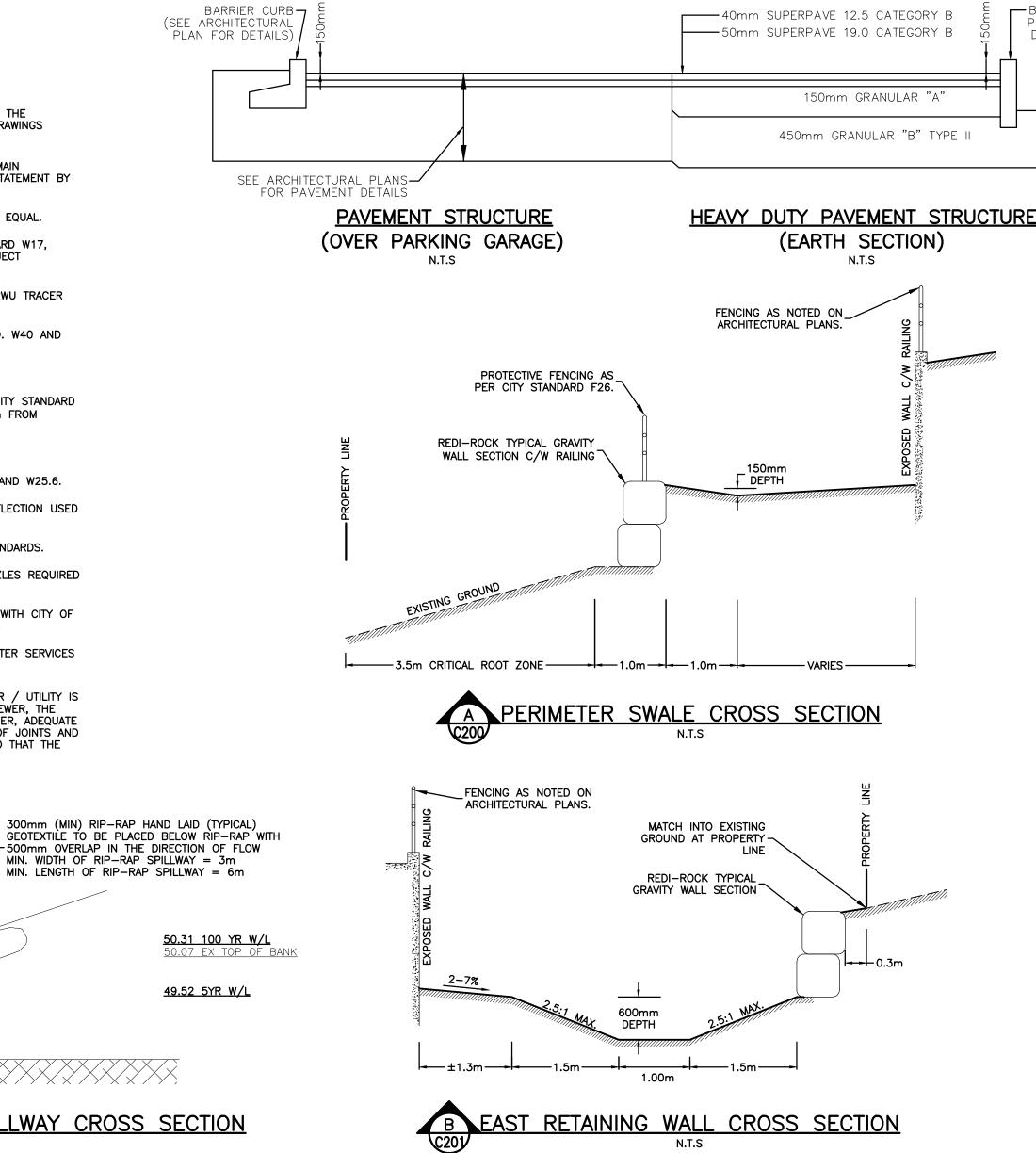
HEAVY DUTY PAVEMENT STRUCTURE FOR NEW ACCESS LANES OVER EARTH SHALL BE AS FOLLOWS: 40mm HL-3 OR SUPERPAVE (PG) 58-34 12.5 ASPHALTIC CONC 50mm HL-8 OR SUPERPAVE (PG) 58-34 19.0 ASPHALTIC CONC. 150mm BASE - OPSS GRANULAR A CRUSHED STONE 400mm SUBBASE - OPSS GRANULAR B TYPE II SUBGRADE - EITHER FILL, IN SITU SOIL OR OPSS GRANUALR B TYPE I OR II
