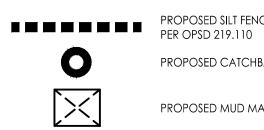
PROPOSED SILT FENCE BOUNDARY AS PROPOSED CATCHBASIN PROTECTION
