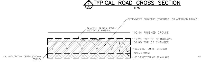
TYPICAL STORM CHAMBERS - CROSS SECTION (SHOP DWGS TO BE PROVIDED BY MANUFACTURER)
