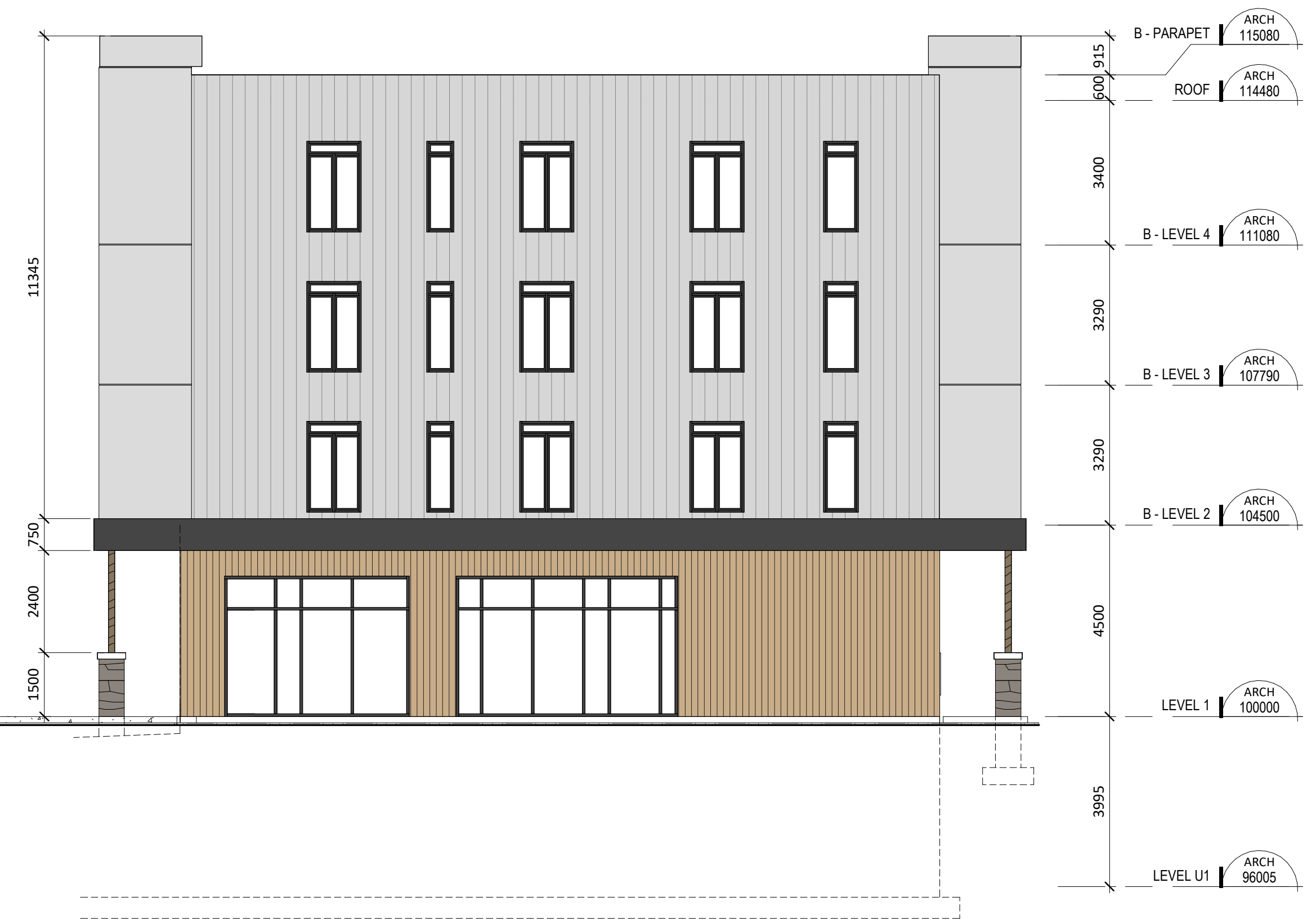
3 LEFT ELEVATION - BUILDING B A303 1:100
