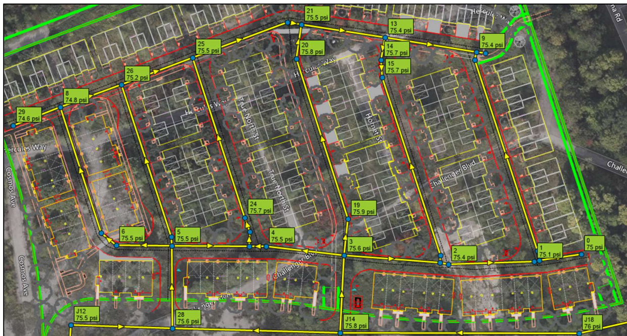
Figure 3.2: Minimum Pressures During PKHR Conditions
