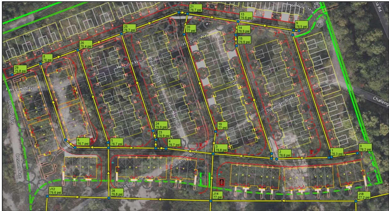
Figure 3.1: Maximum Pressures During AVDY Conditions
