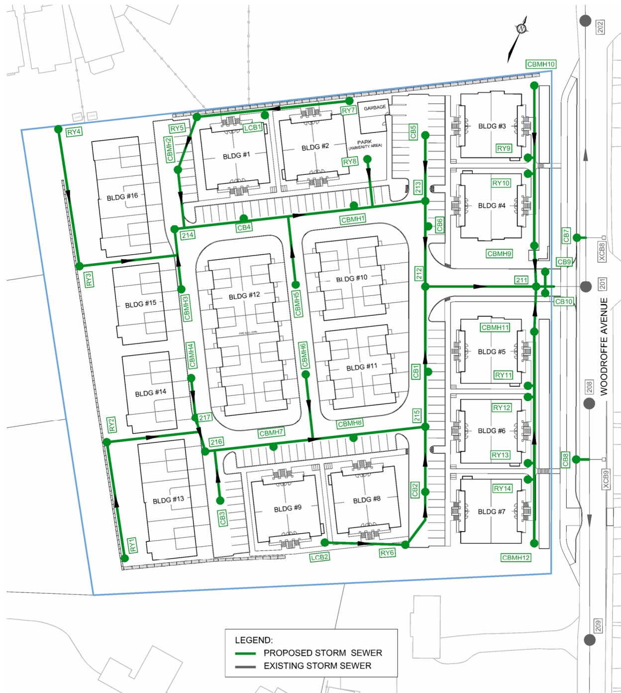
Figure 5: Storm Sewer Network
