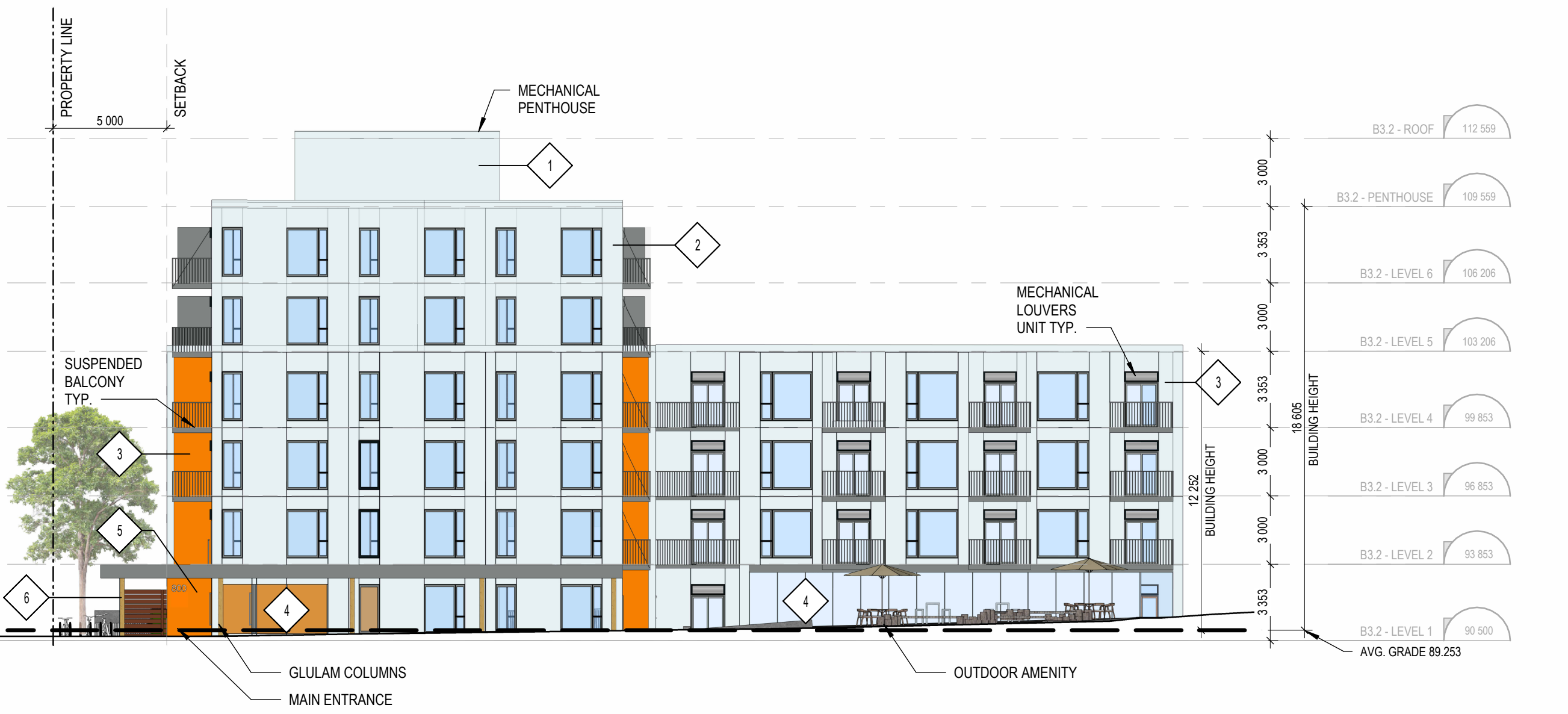
1 BUILDING D - SOUTH ELEVATION A.201 ÉCHELLE / SCALE: 1:200
