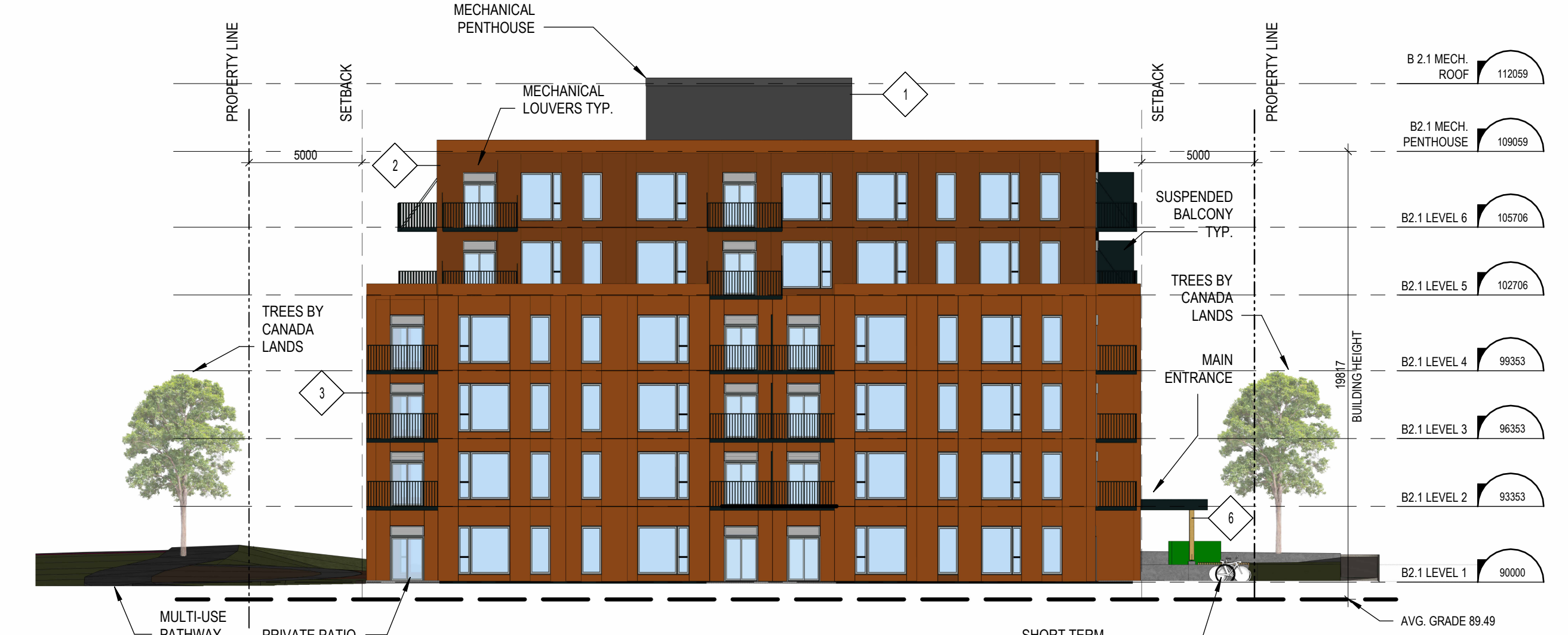
1 BUILDING B - SOUTH ELEVATION ÉCHELLE / SCALE: 1:200 A.201
