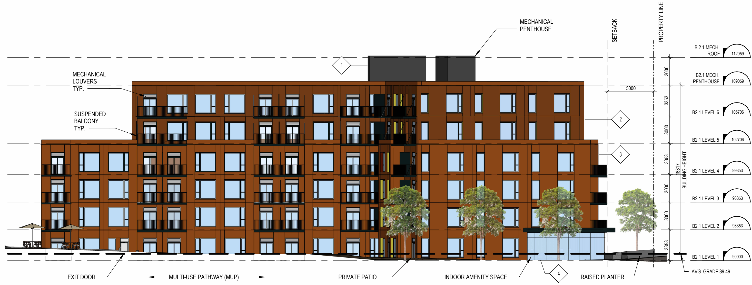
2 BUILDING A - WEST ELEVATION ÉCHELLE / SCALE: 1:200
