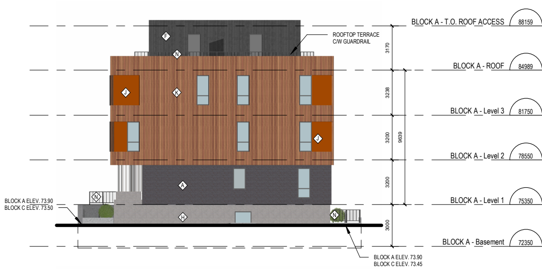
BLOCKS A & C - SOUTH ELEVATION
