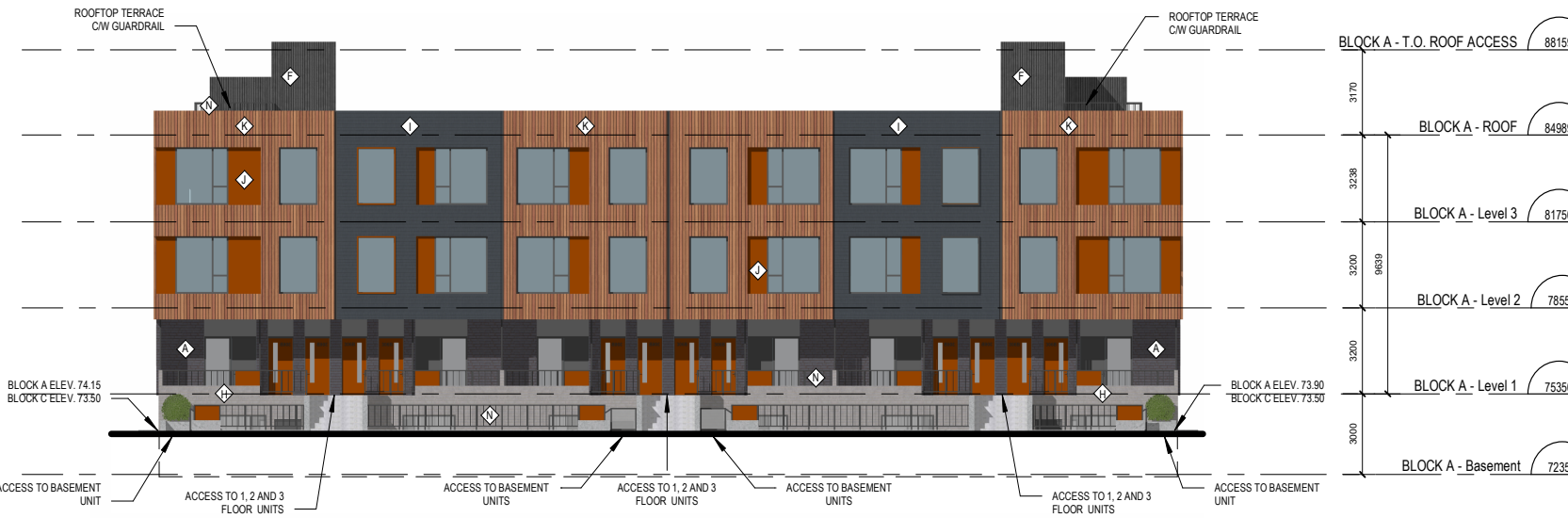
BLOCKS A & C - WEST ELEVATION
