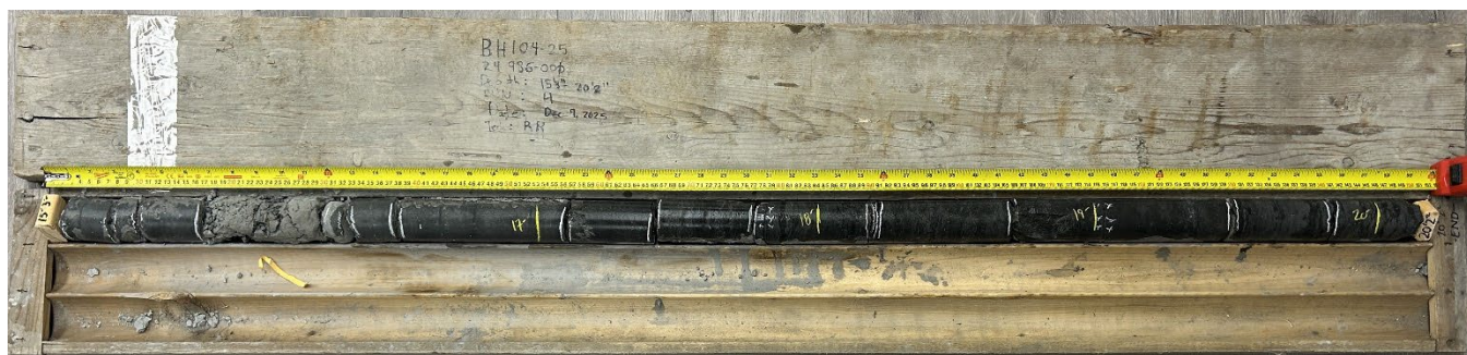
Borehole BH104-25 Rock core run 4.7 to 6.1 mbgs
