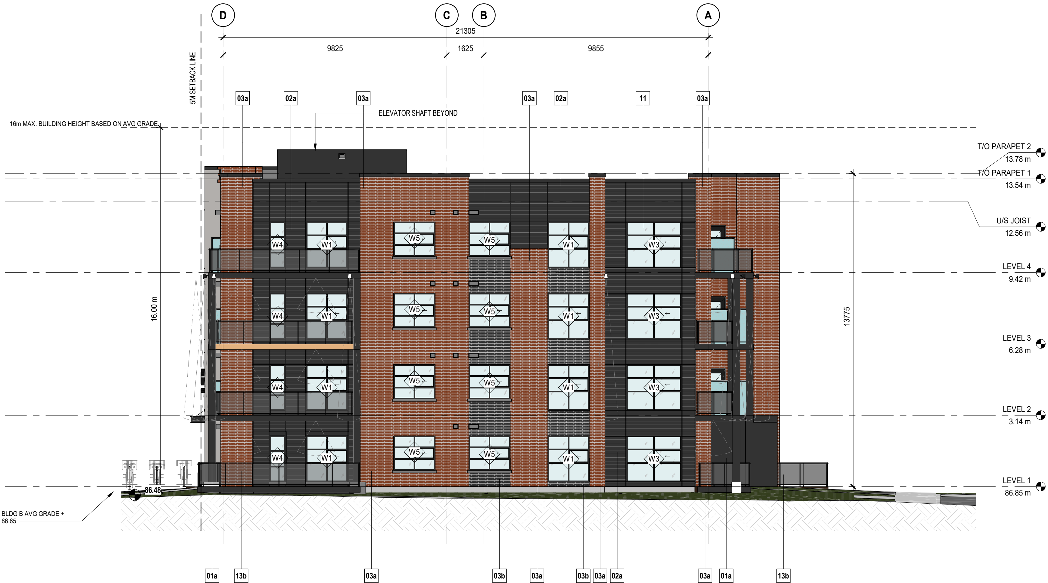
1 NORTH ELEVATION - BUILDING B SCALE: 1: 100
