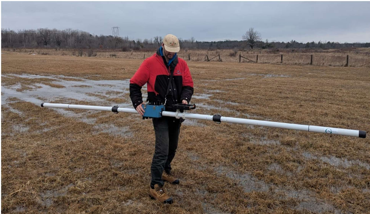
Figure 2: Geonics EM-31 Mk2 on site
