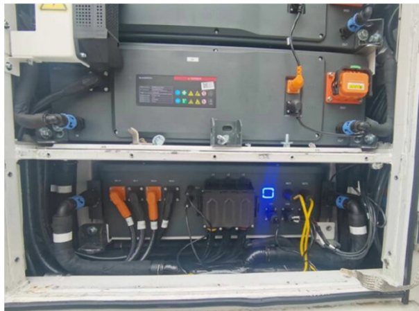
figure 3-3 SCC and BSP Auxiliary Power Supply
