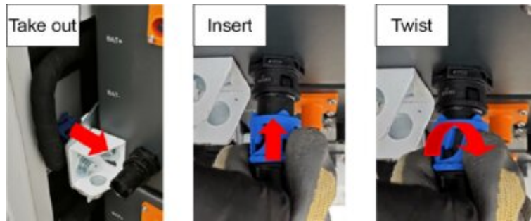
figure 5-26 Installation of Bidirectional Shut-off Valve (Left Side)
